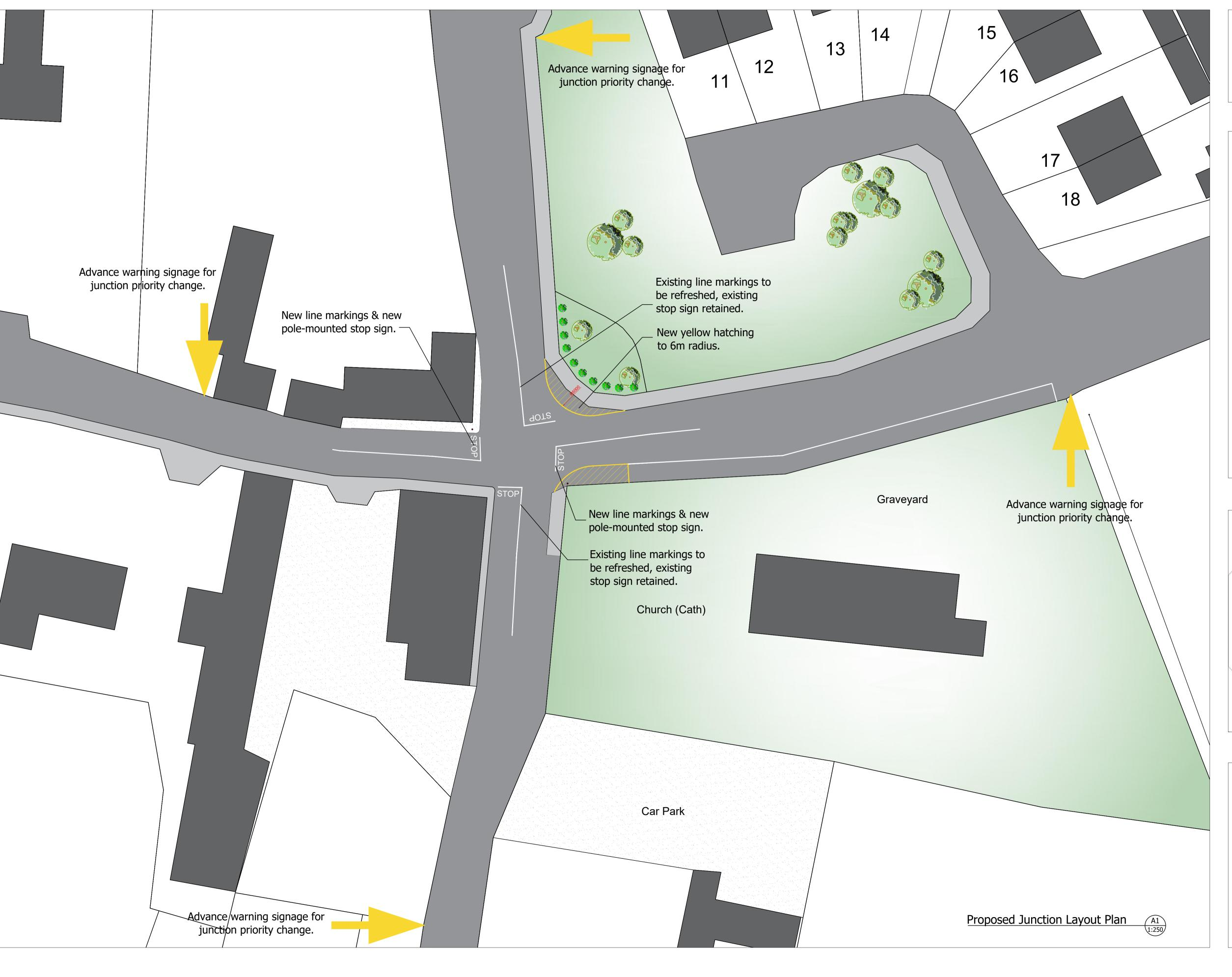
**Advance Warning Signage** to be erected. Engineer to set out sign location. Sign Clearance 2100mm from GL.
